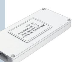
This component is designed for use within the C -band release of DWDM system. To decrease the power dissipation of the devices in different environmental conditions, the AWG package is special designed with selection of reliable thermal plastic with low thermal conduction, and the AWG operating temperature is controlled by using foil resist heater with thermistor temperature sensor.
