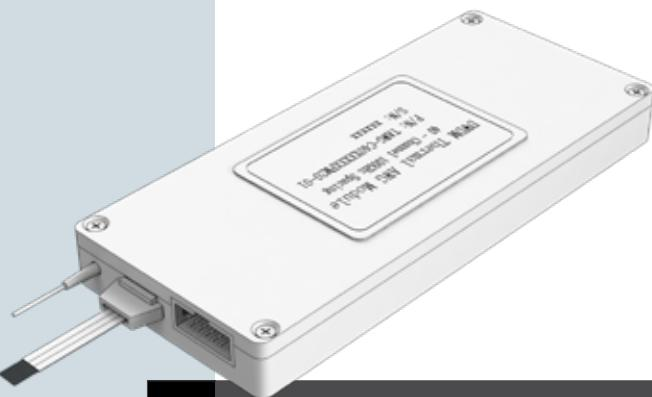
This component is designed for use within the C -band release of DWDM system. To decrease the power dissipation of the devices in different environmental conditions, the AWG package is special designed with selection of reliable thermal plastic with low thermal conduction, and the AWG operating temperature is controlled by using foil resist heater with thermistor temperature sensor.
